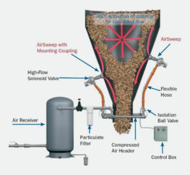
For the initial trial, two bins (9 feet wide, with 200-ton capacity) were hooked up to the **AirSweep VA-12 model 1 <sup>1</sup>/<sub>2</sub> size Four AirSweep** were installed on each bin cone:
