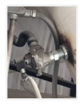
VA-12 Airsweeps® installed on the first bin for initial trial
