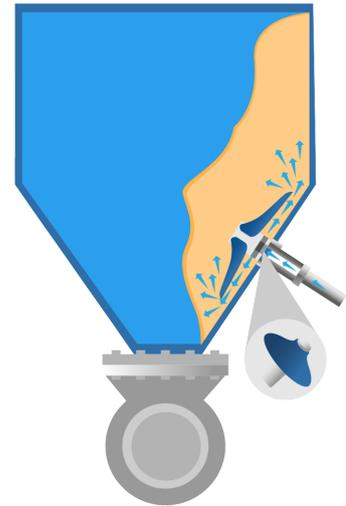
*Fluidizers are a pneumatic flow aid that use a combination of aeration and gentle vibration to promote material flow.*
