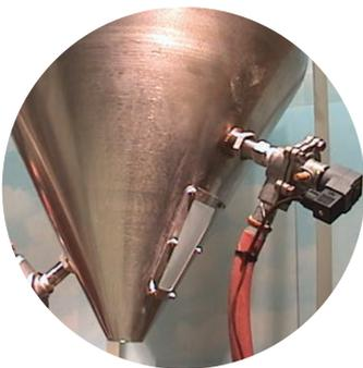
[Two AirSweep VA-06 food-grade units](#) were installed 180 degrees apart, 1.5 feet above the hopper outlet. Special couplings mounted the units to the hopper’s curved surface.
