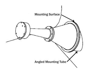
B. Mounting surface sandwiched between bell sections - The horn is mounted such that the end of the last or middle bell section protrudes inside the vessel.
